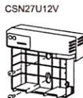
Step 3: a. Use the enclosed installation template to mark an installation location for the unit. b. Mount the unit on the wall with 2 mounting screws into the keyhole slots. c. Tighten the screws to secure the units. d. Connect the battery connector and replace the battery back.
